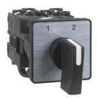
Cam changeover switch, Harmony K, multifixing, plastic, 2 poles, 2 positions, 30°, 12A, 45x45mm, metallic legend, marked 1/2, 35mm black handle
