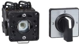
Cam ammeter switch, Harmony K, 22mm, plastic, 3 positions, position 0, 90°, 12A, 45x45mm, metallic legend, marked 0 L1 L2 L3, 35mm black handle
