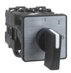
Cam ammeter switch, Harmony K, multifixing, plastic,3 positions, position 0, 90°,12A, 45x45mm,metallic legend,marked 0 L1 L2 L3, 35mm black handle
