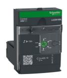
Advanced control unit, TeSys Ultra, 3P, 0.35 to 1.4A, 690VAC, protection & diagnostic, class 10, 24VDC coil
