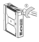
Pivot the module forwards and disengage the pins from the holes located inthe bottom of the support.
