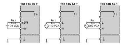
NOTE: When using several ventilation modules of the same type, use a common power supply for all the ventilation modules.
