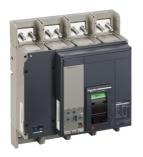
circuit breaker ComPact NS1600N, 50 kA at 415 VAC, Micrologic 5.0 trip unit, 1600 A, fixed,4 poles 4d
