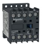
Contactor, TeSys K, 3P, AC-3/ AC-3e,440V 9A, aux. 1NO, 24V AC coil, screw clamps
