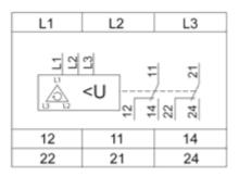
L1,L2,L3 : Supply to be monitored 11-14,12 : 1st C/O contact of output relay 21-24,22 : 2nd C/O contact of output relay
