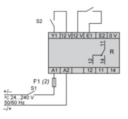
(2) A quick-blow fuse or circuit-breaker.S2 Inhibit - ResetNamur proximity sensor input
