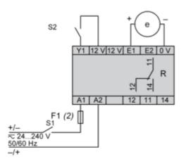
(2) A quick-blow fuse or circuit-breaker.S2 Inhibit - Reset
