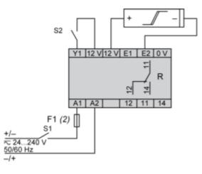
(2) A quick-blow fuse or circuit-breaker.S2 Inhibit - ResetNPN/PNP sensor input
