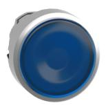
Head for illuminated push button, Harmony XB4, metal, blue flush, 22mm, universal LED, spring return, plan lens, unmarked
