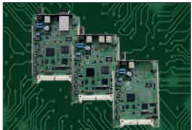
Figure B1.7: Circuit board for numerical relay
