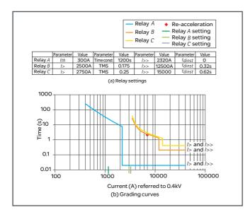
Figure B3.25: Final relay grading curves
