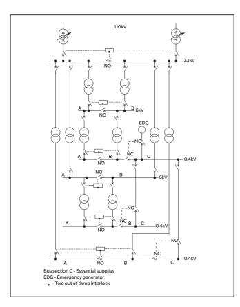
Figure B3.3: Typical industrial power system
