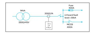
Figure B3.21: Network diagram for protection co-ordination example – fuse/MCCB/relay
