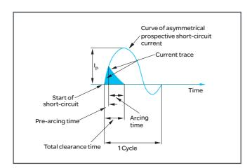
Figure B3.4: HRC fuse cut-off feature
