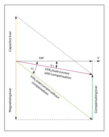
Figure B3.14: Power factor correction principle
