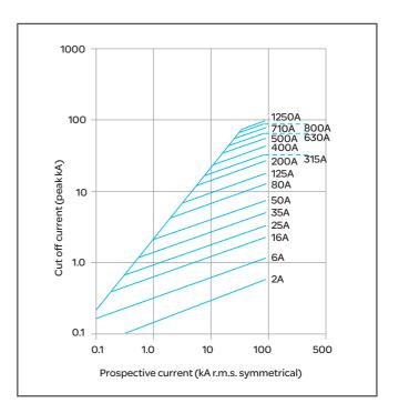
Figure B3.5: Typical fuse cut-off current characteristics
