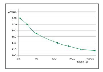
Figure B3.18: Capacitor bank overvoltage characteristic
