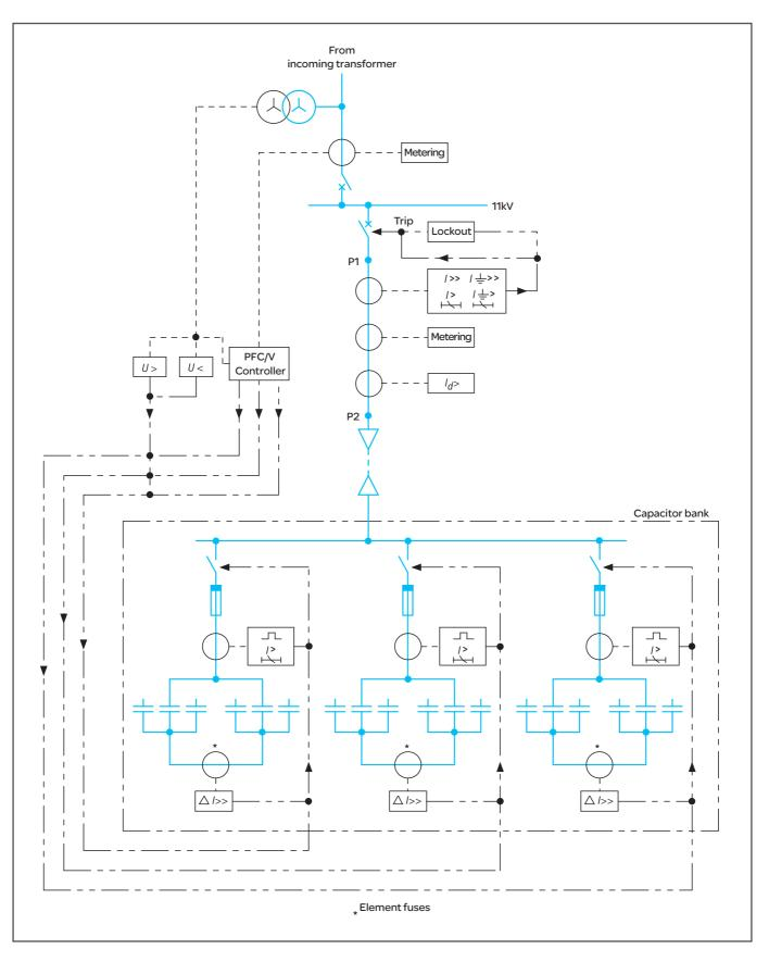
Figure B3.15: Protection of capacitor banks
