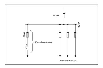
Figure B3.20: Example of back-up protection
